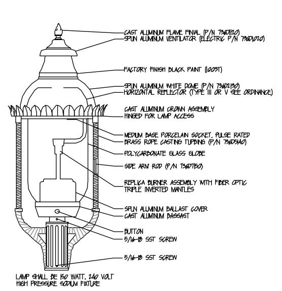
LIGHT FIXTURE SHALL BE MANUFACTURED BY THE PENNSYLVANIA GLØBE GASLIGHT COMPANY, 300 SHAW ROAD, NORTH BRANFORD, CT 06471. (203)484-7749. MODEL "BOULEVARD" OR APPROVED EQUAL. ALL OTHER INSTALLATION REQUIREMENTS SHALL CONFORM WITH THE NORTHAMPTON TOWNISHIP ORDINANCES.
